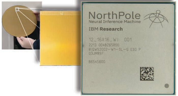
Fig. 3: NorthPole processor: Silicon wafer (left), bare die (center), packaged module (right).
