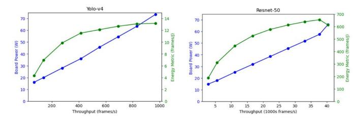
Fig. 4. Measured NorthPole VPX board power, throughput, and energy efficiency. *Left*: Running Yolo-v4 at 350 MHz, the board processed 969 fps at 640 × 640 pixels per image, consuming 73.5 W for a board-level efficiency of 13.2 frames/J. *Right*: Running ResNet-50 at 400 MHz, the board processed 40, 340 fps at 224 × 224 pixels per image, consuming 65.9 W for a board-level efficiency of 612 frames/J.
