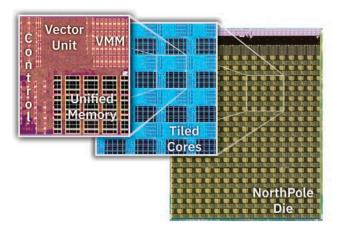
Fig. 3. NorthPole chip micrograph. Each NorthPole core (left) has a vector-matrix multiplication (VMM) unit, a vector unit, unified memory, and control logic. Cores are tiled (middle) in a  $16 \times 16$  array on the NorthPole die (right).
