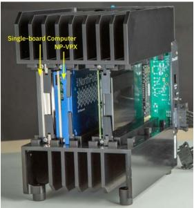
Fig. 1. *Top*: Exploded-view rendering of NorthPole VPX assembly. *Bottom*: Photo of the fully functional, fabricated, and assembled NorthPole VPX module, inserted into a VPX chassis with a single-board computer.
